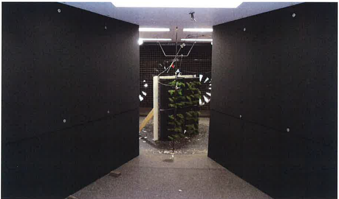
Figure 3b Wind angle of 45 degree (with x axis) set up
