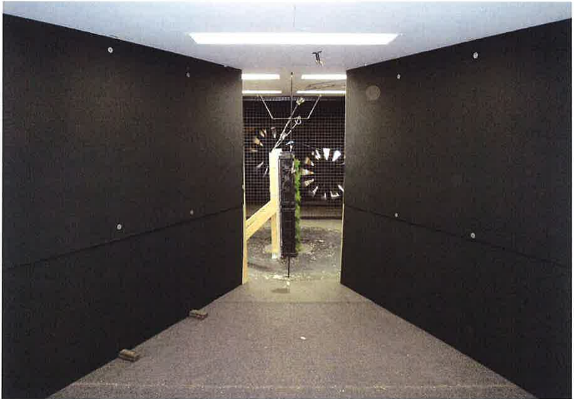
Figure 3a Wind angle of 0 degree (with x axis) set up.
