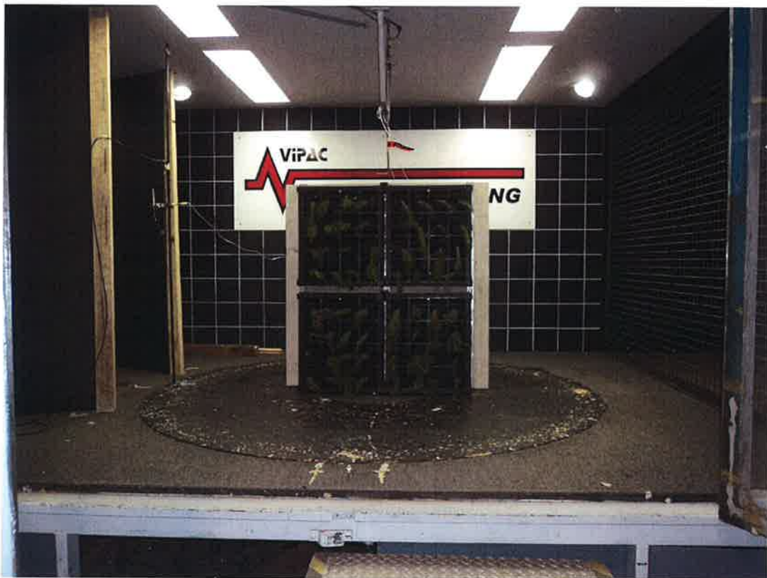
Figure 1 Test sample mounted on the wind tunnel turntable.
